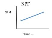
**Upward trend indicates membrane damage**
