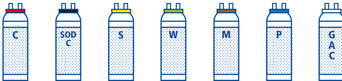
Red Strong Acid Cation (H + Form) Black Strong Acid Cation (Na + Form) Yellow Strong Base Anion (OH - Form) Green Weak Base Anion (Free Base Form) Brown Mixed Bed Blue Mixed Bed Polisher Clear GAC Granular Activated Carbon
