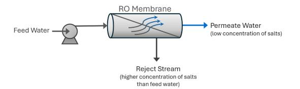
As the feed water enters the RO membrane under pressure (enough to overcome osmotic pressure) the water molecules pass through the semi-permeable membrane and the salts and other contaminants remain on the other side and are discharged from the system through the concentrate stream.
